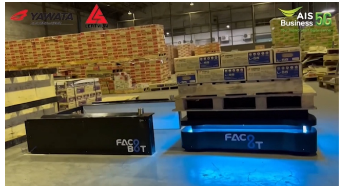
Fig 8. AMR (Automatic Mobile Robot) working with 5G
